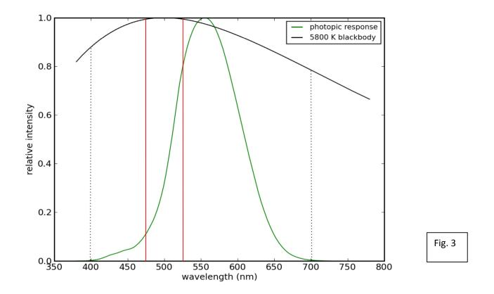
Looking at the two red lines we see that the optimum is between ~475 and 525 nm, this is in the cool blue to greenish area. Monochrome "white like" LEDs are most efficient the in cool blue area.
